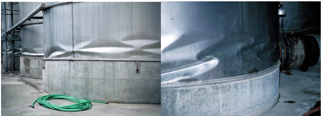
Figure B.5-6 – Diamond-shaped buckling. Livermore (California) earthquake in 1980, M 5.9.
